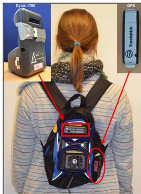
Fig. 1. The monitoring pack – the Dylos monitor is strapped onto the backpack with the inlet (red square) and fan exposed to the air. The GPS is placed in the side mesh pocket.
