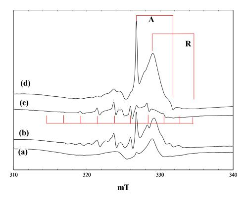
**Figure 2.** EPR spectra of P25 titania in a solution of pivalic acid in acetonitrile at 4 K. (a), During irradiation with low intensity 400 nm light; (b), during irradiation with high intensity 400 nm light; (c), during irradiation with high intensity broad band light; (d), after stopping irradiation.
