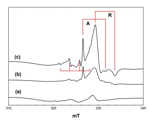
**Figure 1.** EPR spectra of P25 titania in acetonitrile at 4 K. (a), Prior to irradiation; (b), during irradiation with high intensity broad-band light; (c), after stopping irradiation.
