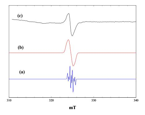
**Figure 5.** Comparison of simulated and observed spectra of the maleimide radical anion. (a), Simulated with a(N) = 0.262 mT, a(2H) = 0.580 mT, a(NH) = 0.031 mT, Gaussian line width of 0.2 mT; (b), Gaussian line width of 0.6 mT; (c), observed spectrum following broad-band irradiation at 80 K.
