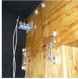
Figure 9. Monitoring knee rotations with “portal” strain gauges.
