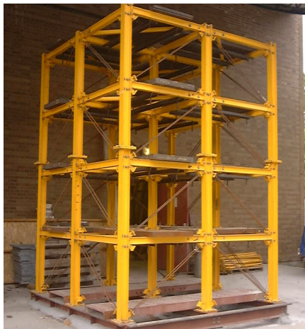
Figure 4. ASCE Phase II Experimental SHM Benchmark Structure.
