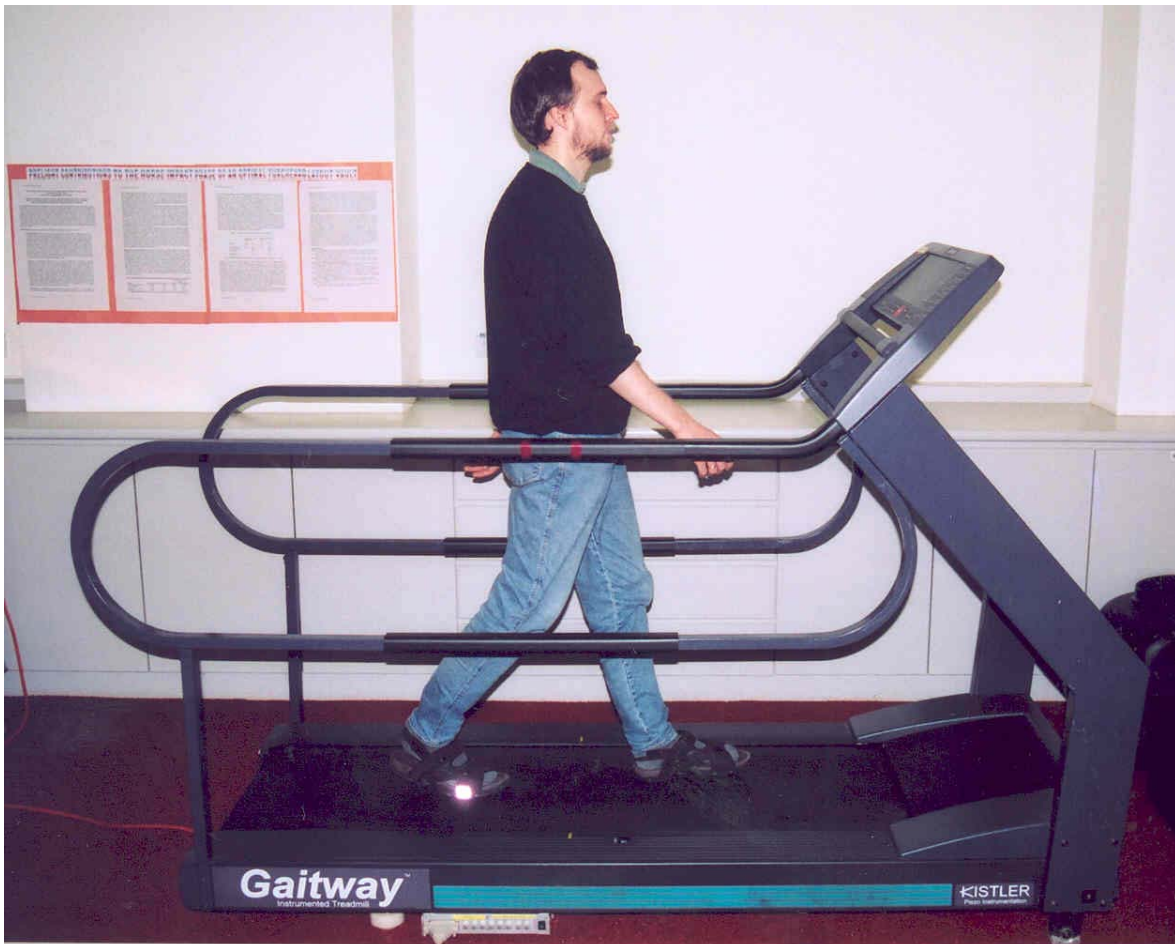
Figure 2: Measurements using Gaitway instrumented treadmill. A fluorescent marker is visible on the right foot of the test subject.
