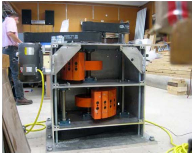
Figure 5. Eccentric mass shakers: a) anchored to the bridge deck (shaker in the front is for vertical and shaker at the back is for lateral excitation), and b) inside of shaker showing rotating masses on flywheels.
