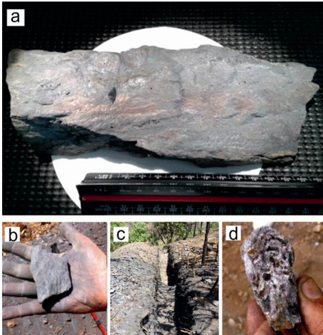
Fig. 6 (a) Hand specimen sample of the (heavily mineralized) quartz-graphitic schist; and (b)-(d) field examples, including (b) a hand specimen showing the high carbonaceous content; (c) outcropping schist (trench excavation) and (d) a sericitic vugge sample.
