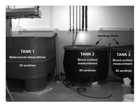
**Fig. 2** Set-up of experimental tanks in the laboratory, including the square-shaped tank used for behavioural observations (*on the left*) and the two round stocking tanks (*on the right*) used for physiological experiments.
