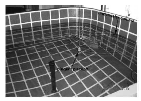
**Fig. 3** Set-up of tank for the behavioural experiments. The position of the underwater camera and the pinger/placebo in the tank are indicated by the arrows.
