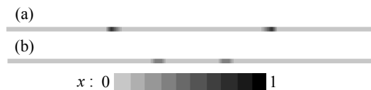
Figure 3. Optimal spring stiffness values for the beam reinforcement problem using a single mode with a) no tracking, b) tracking.
