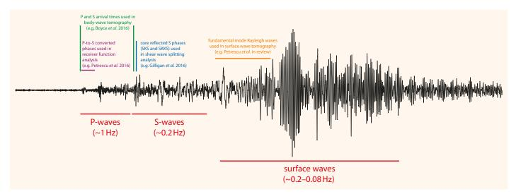
6 Vertical component seismogram from the M7.8 Nepal earthquake of 25 April 2015 recorded at the QM-III station in the museum on Grand Manan Island in the Bay of Fundy. At a distance of 11 200 km, the P-waves arrive after about 25 minutes, the S-waves after about 36 minutes and the surface waves after about 1 hour.
