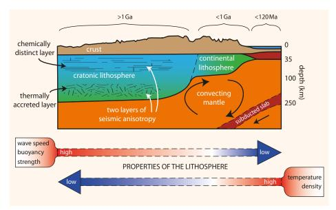
**1** A cartoon summarizing the properties and processes in cratons in relation to other parts of continental plates. The properties wave speed, buoyancy, strength, temperature and density of the lithosphere vary as indicated by the arrows, decreasing from red to blue.
