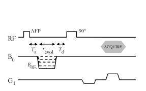
Figure 1: 1D T<sub>1</sub> dispersion pulse sequence
