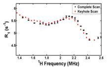
Figure 1: Dispersion curves for a phantom of cross-linked BSA obtained using the keyhole method (red diamonds) show good agreement with results obtained using a conventional field-cycling spinecho sequence (black circles).
