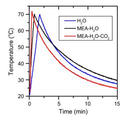
Fig. 2. Microwave heating (100 W) to 70  $^{\circ}$ C and cooling profiles of the different components of the CO<sub>2</sub>-MEA-H<sub>2</sub>O system with 100 mL/min N<sub>2</sub> purge.
