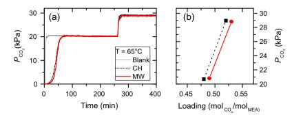
Fig. 4. (a) The CO<sub>2</sub> outlet concentrations versus time for the absorption isotherm measurements at 65 °C for microwave (MW) and conventional heating (CH). The initial inlet CO<sub>2</sub> partial pressure of 20 kPa was increased to 29 kPa after sufficient equilibration time. (b) Equilibrium CO<sub>2</sub> loadings and outlet partial pressures from the isotherm measurements.
