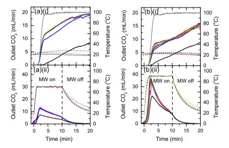
**Fig. 5.** Breakthrough curves (solid lines) and temperatures (dashed lines) for six back-to-back absorption-desorption cycles using microwave regeneration. (a) Regeneration at 70 °C. (b) Regeneration at 90 °C. (i) Absorption step. (ii) Desorption step. Cycle number: 1 (black), 2 (blue), 3 (red), 4 (green), 5 (magenta), 6 (dark yellow). (For interpretation of the references to colour in this figure legend, the reader is referred to the web version of this article.)
