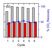
**Fig. 6.** Rich (grey bars) and lean (red bars) CO<sub>2</sub> loadings for (a) 70 °C regeneration cycles and (b) 90 °C regeneration cycles. The percentage CO<sub>2</sub> recovered between the absorption and desorption steps are shown as blue points. (For interpretation of the references to colour in this figure legend, the reader is referred to the web version of this article.)
